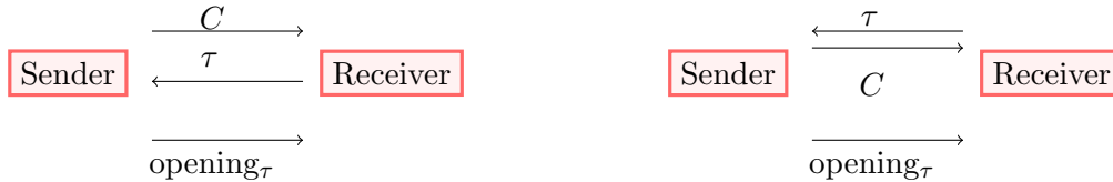
Figure 1: The diagram on the left depicts the communication pattern of Khurana’s [Khu21] commitment scheme, whereas the diagram on the right depicts ours. The key difference is that in our scheme, the receiver’s message and the sender’s messages can be sent simultaneously, while in [Khu21] the receiver’s message must be sent after the sender’s message.
