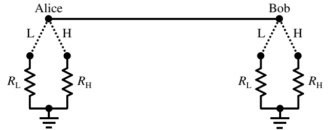
FIG. 1. Basic KLJN protocol. Alice and Bob are at opposite ends of an ideal transmission line, with Eve somewhere in the middle. At each clock cycle Alice and Bob decide independently and randomly whether to terminate their end of the line with a low resistance (L) or a high resistance (H). The Johnson-Nyquist noise from these thermal resistances R_L and R_H at temperature T can be modeled as an ideal resistor in series with a voltage source undergoing Gaussian fluctuations. After transients resulting from this switching have died down, the mean square noise voltage will be the same at any point between Alice and Bob, having one of three values: low (for the LL combination), high (for the HH combination) and intermediate (for LH or HL). Alice and Bob discard data from the HH and LL events, and keep the HL and LH data. The kept events are candidates for a secret key because, knowing their own switch settings, they can distinguish HL from LH, but Eve cannot do so from the mean square noise voltage on the transmission line.
