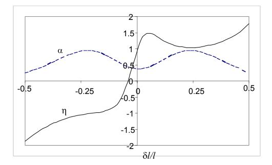
FIG. 16.  $\eta$  ratio (solid line) and signal amplitude  $\alpha$  (dashed line) vs.  $\delta l/l$  for the Continuous Interferometer, simulated with parameters  $\Omega_0 = 2\pi (7 \times 10^4)$ , L = 3 × 10<sup>-3</sup> m.,  $\Omega_0 T = 3.3$ . The signal amplitude is symmetric around  $\delta l = 0$ , and reaches a maximum at  $\delta l = \pm 12/25$ . At these values the interferometer behaves most like a BCI, with the effective area also leveling off temporarily before increasing.
