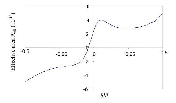
FIG. 13. Effective area (m<sup>2</sup>) vs.  $\delta l/l$  for Continuous Interferometer, simulated with parameters  $\Omega_0 = 2\pi (7 \times 10^4)$ , L = 3 × 10<sup>-3</sup> m.,  $\Omega_0 T$  = 3.3. The area for a comparable BCI is 2.7× 10<sup>-10</sup>.
