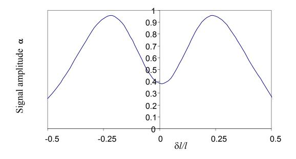
FIG. 12. Signal amplitude  $\alpha$  vs.  $\delta l/l$  for the Continuous Interferometer, simulated with parameters  $\Omega_0 = 2\pi (7 \times 10^4)$ , L = 3 × 10<sup>-3</sup> m.,  $\Omega_0 T$  = 3.3.
