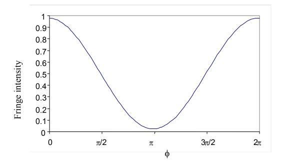
FIG. 15. Phase scan for the Continuous Interferometer when the phase is applied at  $\delta l/l = \pm 12/25$ , giving the maximum fringe contrast most comparable to the BCI. Simulated with parameters  $\Omega_0 = 2\pi (7 \times 10^4)$ , L = 3 × 10<sup>-3</sup> m., v=300m/s,  $\Omega_0 T = 3.3$ .
