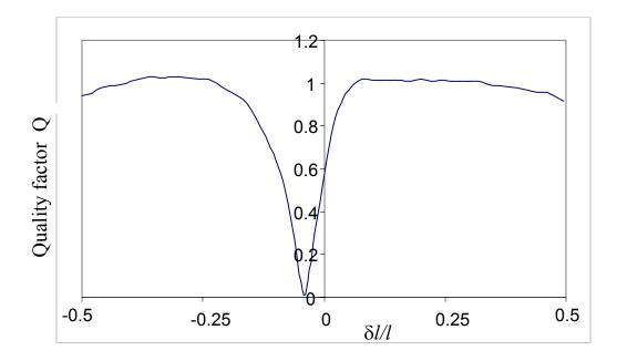
FIG. 14. Quality Factor Q vs.  $\delta l/l$  for the Continuous Interferometer, simulated with parameters  $\Omega_0 = 2\pi (7 \times 10^4)$ ,  $L = 3 \times 10^{-3}$  m.,  $\Omega_0 T = 3.3$ .
