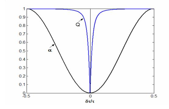
FIG. 5. Typical plots of  $\alpha$  and Q versus  $\delta \tau / \tau$ , for  $\Omega_0 = 2\pi (7 \times 10^4) \text{ s}^{-1}$ ,  $L = 3 \times 10^{-3} \text{ m}$ , and  $k = 8.055 \times 10^6 \text{ m}^{-1}$  (corresponding to the D2 transition in Rb), and  $\delta \phi_0 = 0.1$ . Note that the quality factor never exceeds unity, and drops to zero as  $\delta \tau$  goes to 0.
