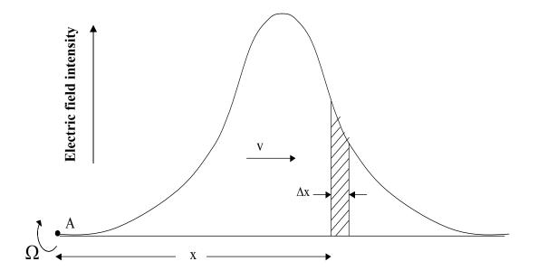
FIG. 6. Electric field intensity profile of counter-propagating laser beams for the Continuous Interferometer. The field intensity of the laser beam varies in the x direction as a Gaussian. The entire setup is rotating around point A, with the atom moving at speed v in the x direction.
