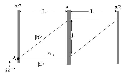
FIG. 2. Schematic of the setup for the Borde-Chu Interferometer. The atom moves at some speed  $v_x$ , with the two atomic states deflected along different paths. The entire system is rotating around point A at some rotational velocity  $\Omega$ .
