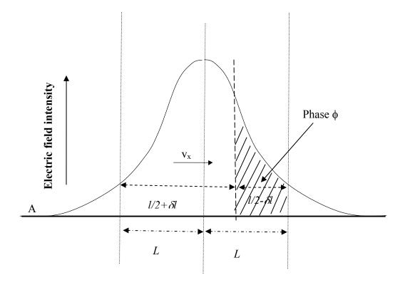
FIG. 7. Phase-shift application in the continuous interferometer (CI). The phase is applied after a distance  $\delta l$  from the middle of the beam as indicated by the shaded region. The velocity of the atom along the x direction  $v_x$  relates L and T:  $L = v_x T$ .
